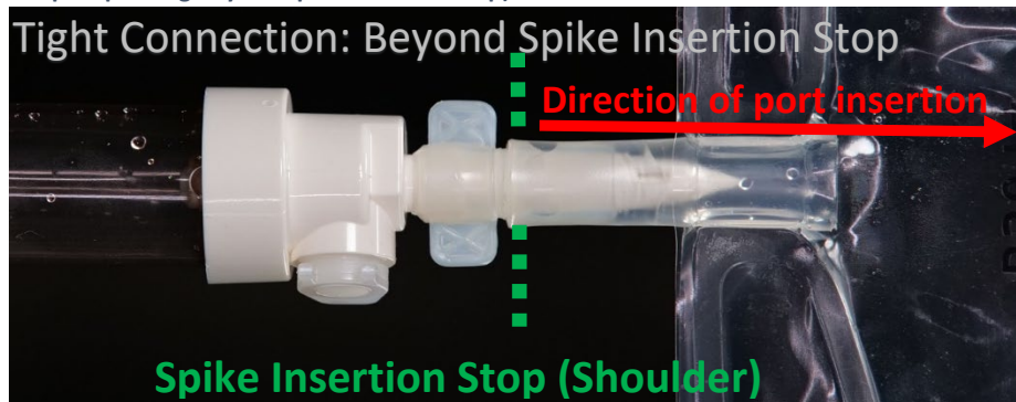
Figure 3: CORRECT spike insertion into the twist off port (piercing device all the way into the port pushing beyond spike insertion stop)
